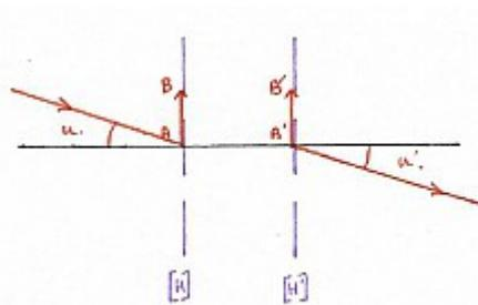
$$\gamma_a \times \gamma = \frac{m}{m'} \quad \gamma = 1 \text{ do ce cas } \gamma_a = \frac{u'}{u}$$
